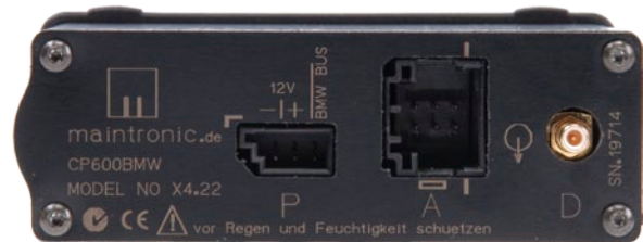
CP600BMW rear view with connectors
