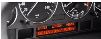
Display at the BMW IKE speed instrument panel
