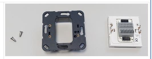
Remove the grey terminal block with PCB from the TS2.
