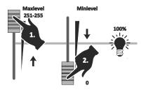
The dimmer accepts this channel as a new DMX start address. This is indicated by two long flashes of the LED and possibly connected lights go to 100% brightness for about one second. Afterwards, the programming mode is exited.
