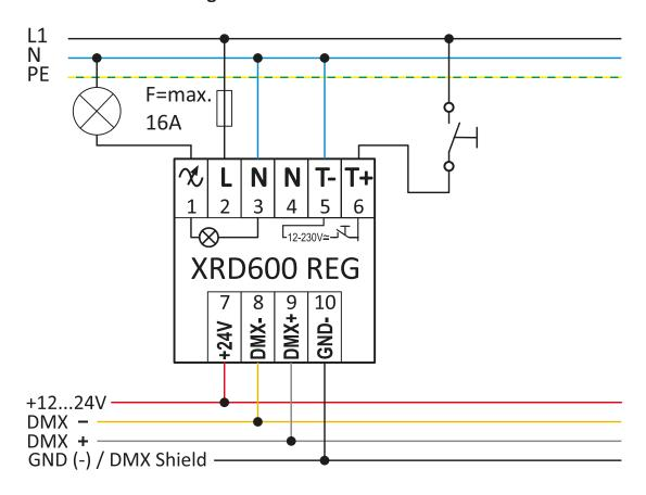
Fig. 2 - Connection diagram with push button 230 VAC
