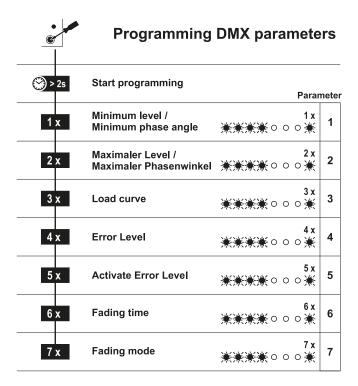
Press the device button > 2 seconds ... (load jumps to 0 and 100% for half a second each), then the LED flashes consistently.
