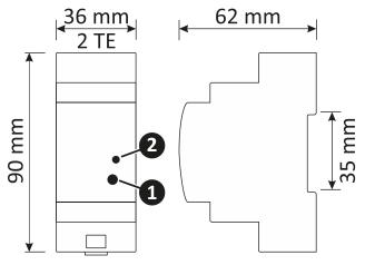
Fig. 1 - Housing dimensions and connections
