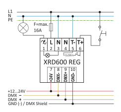
Connection diagram with push button 230 VAC
