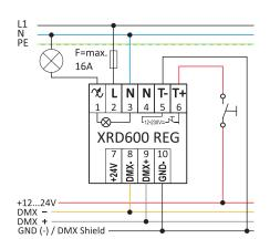
Connection diagram with push button 230 VAC
